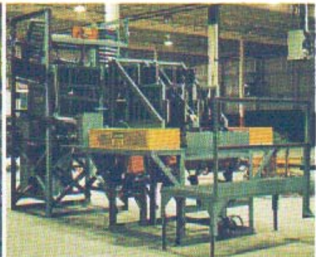
This device was built for the rubber industry for trimming tire vent flashing. Tires are introduced at the top of the unit where they are uprighted and dispatched down one of two lines. The tire is then rotated and the flashing trimmed off. Webb-Stiles has wide conveyor experience in the rubber industry.
