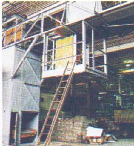
1 of 5 lifts built to overhead conveyors. This system was built for handling air freight in Saudi Arabia. The unit just to the right powers the overhead belt conveyor. This was set-up in our plant for test operating.
