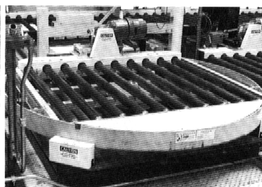
Turntables can be electrically or pneumatically powered to accurately rotate 360 degrees. They can be combined with chain transfers or elevating devices for versatility.
