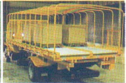
The Transpor-Con transporter truck is equipped with a powered roller conveyor deck that is raised or lowered for alignment with dockside conveyors. The rollers and lift are hydraulically powered by an on-board PTO.
