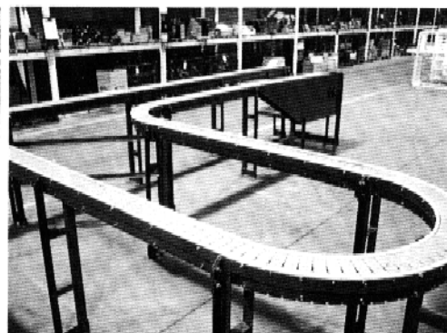
A narrow flat-top hinged slat conveyor for handling gears and trunnions. The slats are made of plastic and are chain driven.
