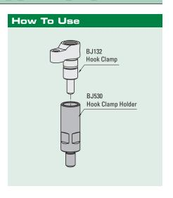
These cylindrical holders are designed for use with the compact hook clamps shown above. They provide additional clamping height as well as easy installation and operation of the hook clamps. Made from SAE-1045 alloy steel, heat treated with black oxide finish.
