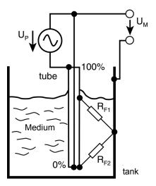
The measuring principle is comparable to that of a slider potentiometer, with in this case the liquid representing the slider pick-off.
