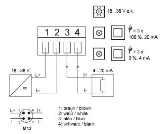
Terminals 1(+) and 2(-) are used for supplying a DC voltage of 18...36 V. Terminal 2 is connected to the housing via a protective diode.
