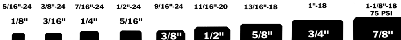
Actual Profile of Compression Threads
