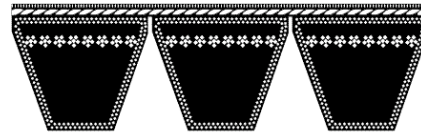
ENVELOPE 5V, 8V CROSS SECTION
