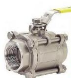
3-Piece Full Port 4-Bolt 316 Stainless Steel Body, Ball & Stem 304 Stainless Steel Handle & Nut
