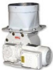
Airlocks maintain a continuous vacuum at the bottom of the cyclone, eliminating the need for an air tight seal between the cyclone and the dust bin. The wood waste continuously drops straight down.
