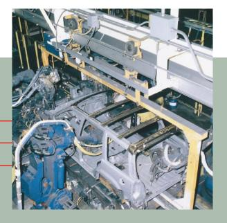
Top right: Automated Electrified Monorails deliver parts to multiple workstations at a high-tech manufacturing facility.
