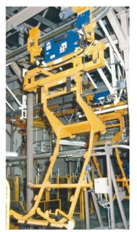
Vertical lift devices used in Webb AEM systems feature double mast structural tube steel construction. Additional features include an electric gear motor, variable frequency drive with Eurodrive Reducer, a standby drive motor, and a separate emergency caliper brake as well as an integral motor brake.
