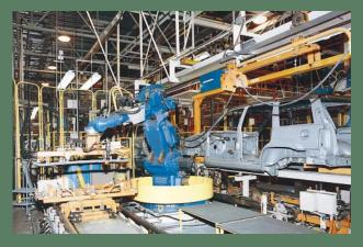
through stations where the engine compartment is mounted and welded to form the underbody.
