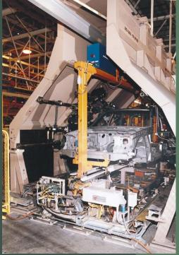
Bi-directional carriers individually powered by track mounted electrification
