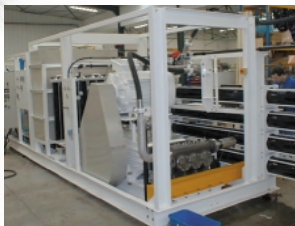
150 Frame Salt Water Reverse Osmosis Systems
