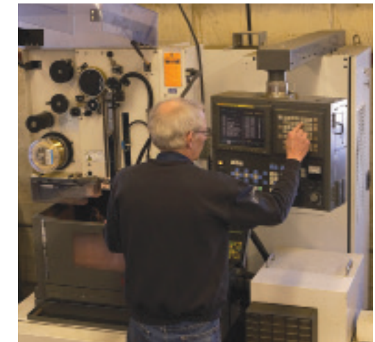
Machinist setting up for a new run at an Eagle wire electronic discharge machining center.
