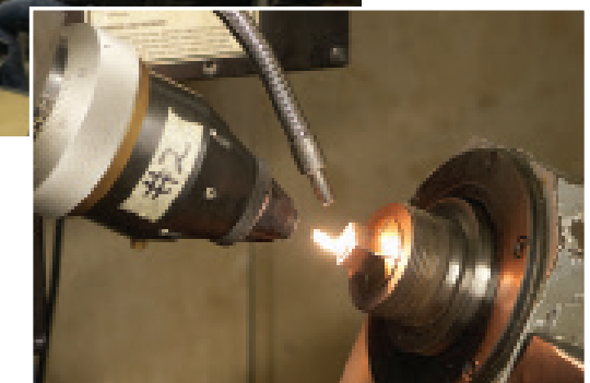
Computer controlled laser machining equipment enables extremely close-tolerance cutting, notching, etching and welding operations. Some assemblies require both laser welding and soldering as shown in the typical drawing below.
