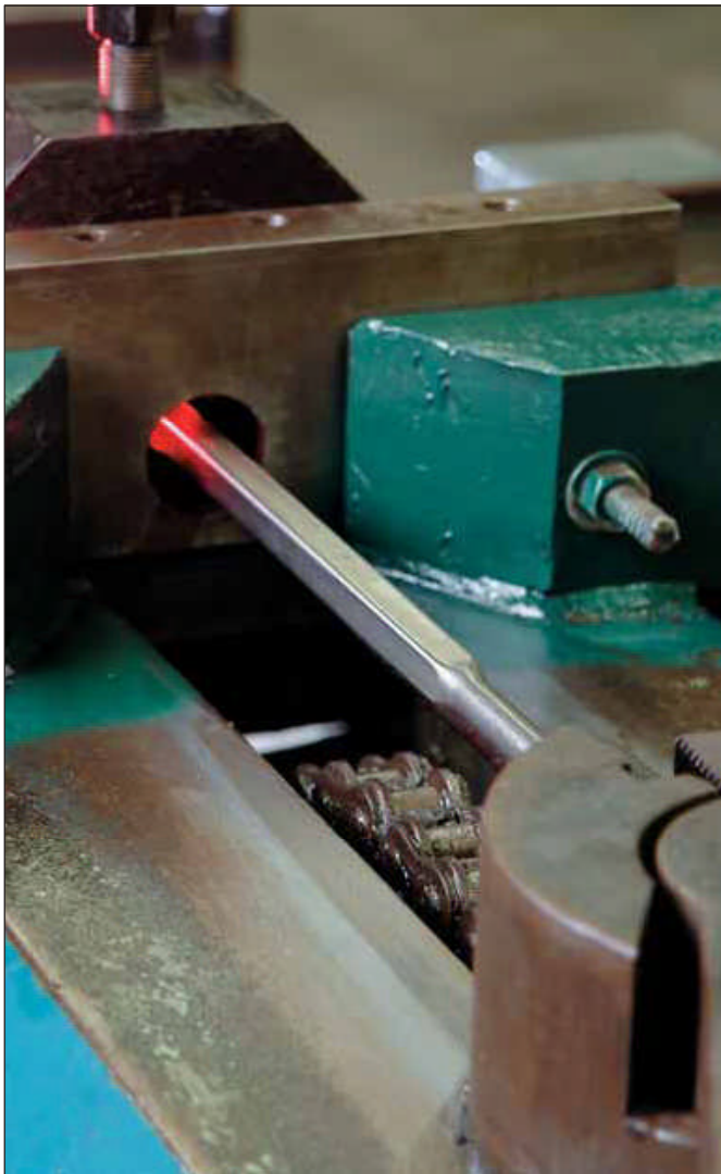
Extrusion dies, designed and built in-house at Eagle, enable a variety of tubing materials to be drawn to precise, unique, custom shapes.
