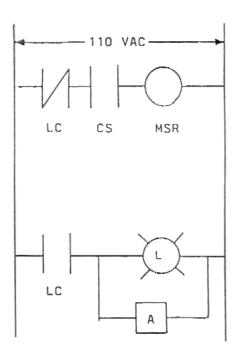
MSR Pump Motor Starting Relay
