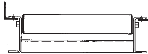
Angle guard, "set-out" type, bolted to underside of top flange of roller conveyor frame.
