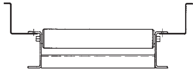
Extended formed metal guard, "set-out" type, bolted to underside of top flange of roller conveyor frame. This type of guard is made to order to satisfy requirements.
