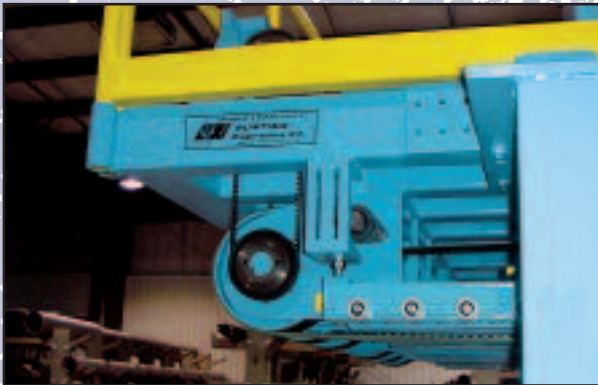
Sheet Stacker Drive (side view)
