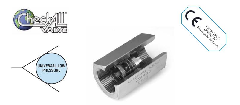
The Universal Low Pressure (U3) check valve is a one piece body machined from bar stock and is designed for minimum pressure drop. The valve has a light weight compact design that provides maintenance-free, dependable service. Threads are per ASME B1.20.1. Also available with ISO 7 "Rp" threads. (UR)
