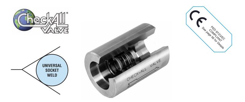
The **Universal Socket Weld (US)** check valve is a one piece body machined from bar stock with socket weld ends and is designed for a minimum pressure drop. It carries rugged, dependable Check-All trim and there are a wide variety of seat materials and cracking pressures to choose from. The socket parts are machined to ASME/ANSI B16.11 dimensions.
