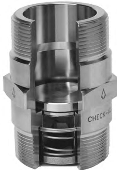
The **Connector (CN, CR)** valve is a check valve with a pipe nipple or connector housing. It is designed to be used in installations where a check valve with male pipe threads is required. The CN valve is adaptable for use as a low pressure relief valve or vacuum breaker by using the desired spring settings. Two valves used in combination make an excellent pressure vacuum vent. NPT threads are per ASME B1.20.1. Also available with ISO 7 "R" threads (CR).
