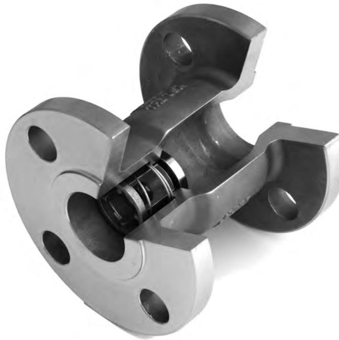
The **Check-All® Flanged & Drilled (HV)** check valve is a one piece cast body valve with ASME/ANSI B16.5 Class 150 flanged ends. The HV series valve is used when higher flow rates and lower pressure drops are required. The valve is available in sizes 1 inch through 10 inches and standard materials of CF8M (cast 316 stainless) and WCB/WCC (cast carbon steel). The HV series valve is designed for use with mating ANSI class 150 flanges. Other materials are available upon request.
