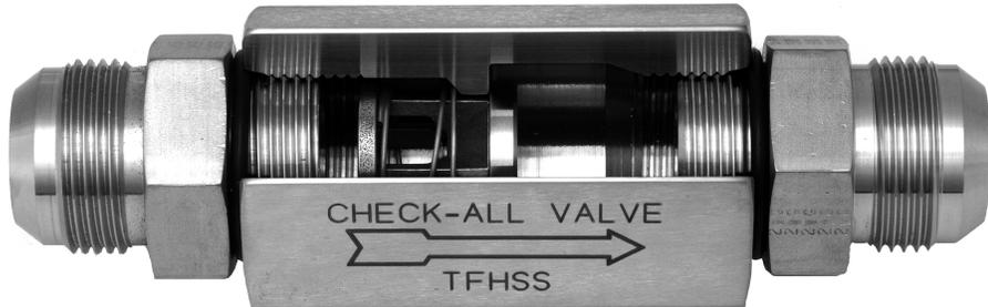
The **Tubing Check Valve-Flared (TF)** is a three-piece constructed check valve with 37° flared end fittings that conform to SAE J514 & ISO 8434-2 . These valves are designed for maximum flow with minimal pressure drop. The TF valve can also be used as a low pressure relief valve or vacuum breaker by using the desired spring settings.
