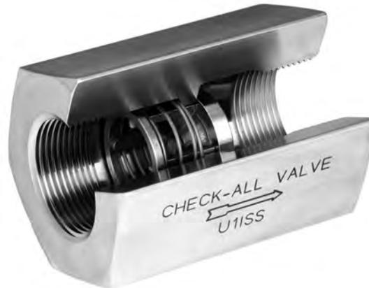
The **Universal High Pressure (U1, R1)** check valve is a one piece body machined from bar stock with female pipe threads. The valve is designed and manufactured for high pressure applications. These valves can also be used as low pressure relief valves or vacuum breakers by using the desired spring settings. This valve is normally supplied with a “metal-to-metal” seat. NPT threads are per ASME B1.20.1. Also available with ISO 7 “Rp” threads. (R1).
