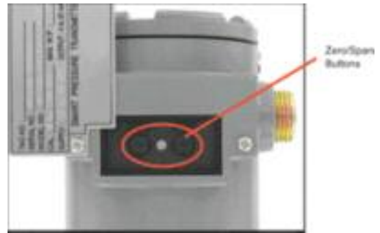
Figure 3-4 Transmitter Zero/Span Configuration Buttons
