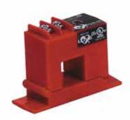
The Series CT40/50 Current Transformers combine a current transformer and a signal conditioner into a single package. Units are designed for applications on linear on sinusoidal loads. Series CT60/70 provide true RMS outputs on distorted AC waveforms — ideal for nonlinear loads or noisy environments. Transformers feature jumper selectable ranges and split-core case.
