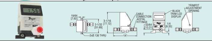
Series TFP-GI Gas Turbine Flow Meters are suitable for a wide variety of industrial, commercial, and laboratory flow applications. These meters utilize a turbine wheel and electro-optical detection to convert flow rates into a linear 0 to 5 VDC output signal for recording and data logging. A 3-1/2 digit LCD informs the user of the actual flow rate. A power adapter or mating cable assembly is required for operation.
