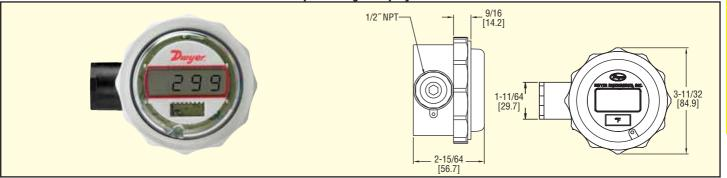
The Series BPI Battery Powered Indicator accepts RTD or Thermocouple input and provides local or remote display of temperature measurements. Quickly navigate the menu system to customize for each application. Three push buttons allow the user to select input type, engineering units (°F or °C), offset temperature, decimal point position, and password protection. The indicator is housed in a polycarbonate NEMA 4X (IP65) enclosure for additional protection from the environment.
