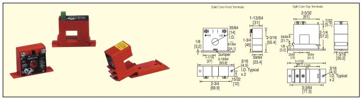
The CS Series Current Switches combine a current transformer, signal conditioner and limit alarm into a single package. The CS series has an extended current input range, universal solid-state outputs and a wide frequency response. Available in a split core or a solid core case. Switches feature LED indication for local display or switch status.
