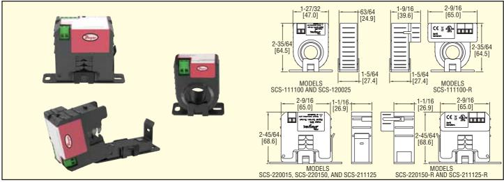
The Series SCS Low Cost Current Switches are ideal for monitoring whether fans, pumps, or motors are operating. The current flowing through the core of the device powers the circuit without an external power supply. All models have a built in solid state output and are easy to install. Optional LED's and 10 Amp relay modules are available. The Series SCS is available in both Split and Solid Core configurations.
