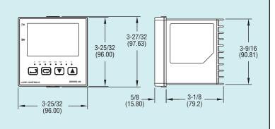
The Series 4B 1/4 DIN Temperature/Process Controller is designed to accept thermocouple, RTD, current or voltage input and provide dual outputs for control. Available outputs include relay/relay, voltage pulse/relay, current/relay, or linear voltage/relay.
