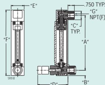
**Series TVA All Fluoropolymer Flowmeters** offer solutions for measuring flow rates of highly corrosive or ultra-pure liquids. Flowmeters are designed with 0 to 10 scale graduations denoting a discrete flow rate.
