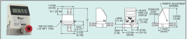
Series TFM-LI Liquid Turbine Flow Meters are suitable for a wide variety of industrial, commercial, and laboratory flow applications. These meters utilize a turbine wheel and electro-optical detection to convert flow rates into a linear 0 to 5 VDC output signal for recording and data logging. A 3-1/2 digit LCD informs the user of the actual flow rate. A power adapter or mating cable assembly is required for operation.
