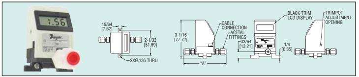
Series TFP-LI Liquid Turbine Flow Meters are suitable for a wide variety of industrial, commercial, and laboratory flow applications. These meters utilize a turbine wheel and electro-optical detection to convert flow rates into a linear 0 to 5 VDC output signal for recording and data logging. A 3-1/2 digit LCD informs the user of the actual flow rate. A power adapter or mating cable assembly is required for operation.
