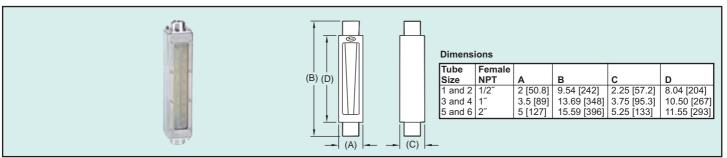
**Ideal for industrial applications**, the Series IF Industrial Direct Reading Flowmeters are fully enclosed in a brushed stainless steel case. The flowmeters can directly measure flow rates up to 116 GPM (439 lpm) for water and 250 SCFM (7080 lpm) for air service. The detachable, clear 3/16" thick polycarbonate front shield provides protection at maximum rated temperature and pressure. Each unit is designed with female NPT end fittings for easy in-line installation.
