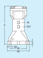
Series APV-C Piston Vibrators are air cushioned to provide low noise. This makes it suitable for quiet area applications. It is a good solution to prevent clogs on tank walls and material delivery problems. It can also be applied on vibrating separators and conveyors.
