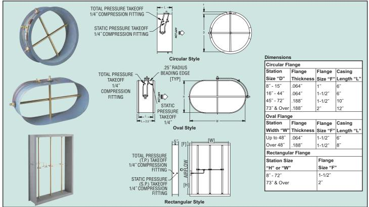
The Series FLST Airflow Measurement Station is easy to install - simply connect the tubing to the station fittings, then to a differential pressure manometer, gage, transmitter or switch. Single or multiple airflow elements are factory mounted and pre-piped in a casing designed for flanged connection to the ductwork. Standard materials consist of a G90 galvanized casing and 6063-T5 anodized aluminum flow sensors, suitable for most HVAC applications.
