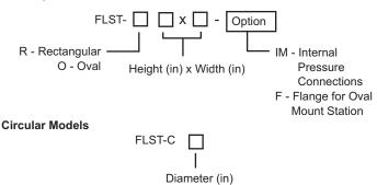
Note: When ordering rectangular or oval flow stations, pressure taps will always be located on the longer of the two dimensions.
