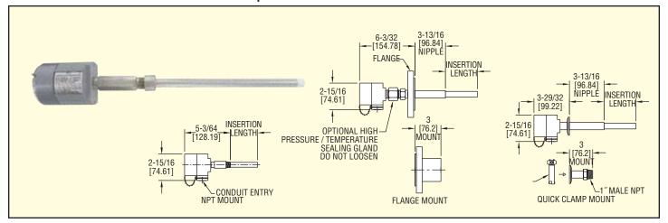
The Series PMT Particulate Transmitter is a reliable dust collector emissions monitor and leak detector. The loop powered design is ideal for direct connection to existing PLCs or other baghouse diagnostic control systems. Adjustable linear or logarithmic output scaling enables trending both the baseline emissions and the high peak emissions that are caused by filter cleaning cycles and developing leaks. Observation of both baseline and peaks is essential to setting proper alarms.
