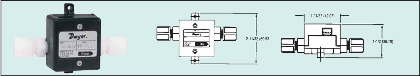
Series TF Turbine Flow Sensors are suitable for a wide variety of industrial, commercial and laboratory flow applications. Sensors use a turbine wheel and electro-optical detection to convert flow rates into a linear 0 to 5 VDC signal for recording and datalogging. Models for use with liquids also provide a pulsed output for flow totalizing – see model TM2 on page 188 for a compatible display.
