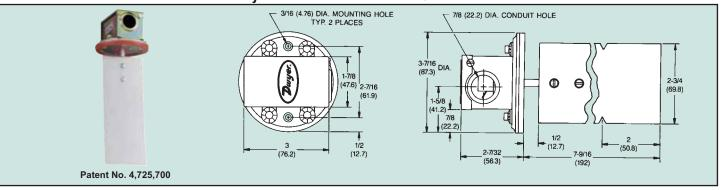
**The Model 530 air flow switch** provides excellent sensitivity and reliability at a very reasonable price. Quality features include a rugged die cast body, stainless steel vane and SPDT snap switch. Unit is field adjustable from 400-1600 FPM. Mounting is fast and simple, with only two screws needed. Vane fits 6 in. or larger ducts.
