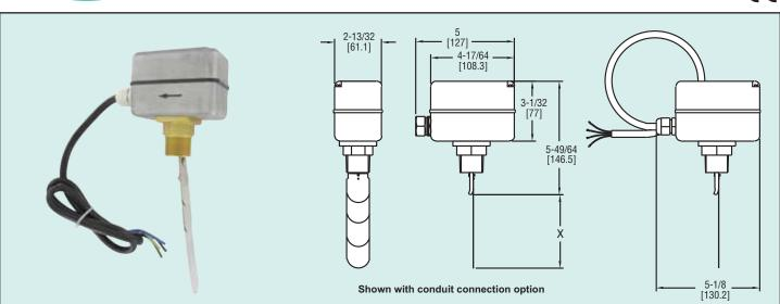
The Series FS-2 Vane Flow Switch offers an economical flow proving solution. Custom set points tailored for the application are enabled by field adjustable vane layers and a set point adjustment screw. The FS-2 features an aluminum weatherproof housing for outdoor installation. Paddles are adjustable to fit 1" to 8" size pipe. FS-2 is ideal for use in "flow or no flow" applications in cold and hot water systems. Perfect for proving flow in boilers, hot water heaters, and chillers.
