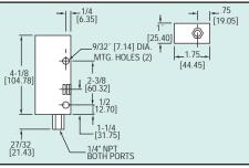
**The Series P1 Brass Flow Switch** utilizes a piston-type design for accurate detection of excessive or insufficient flow rates. The piston magnetically actuates a hermetically sealed SPDT reed switch. The switches have preset actuation points from 0.10 to 1.5 GPM for liquid flow. The Series P1 is ideal for protecting against loss of fluid flow in hydraulic systems or assuring proper coolant flow in semiconductor processing.
