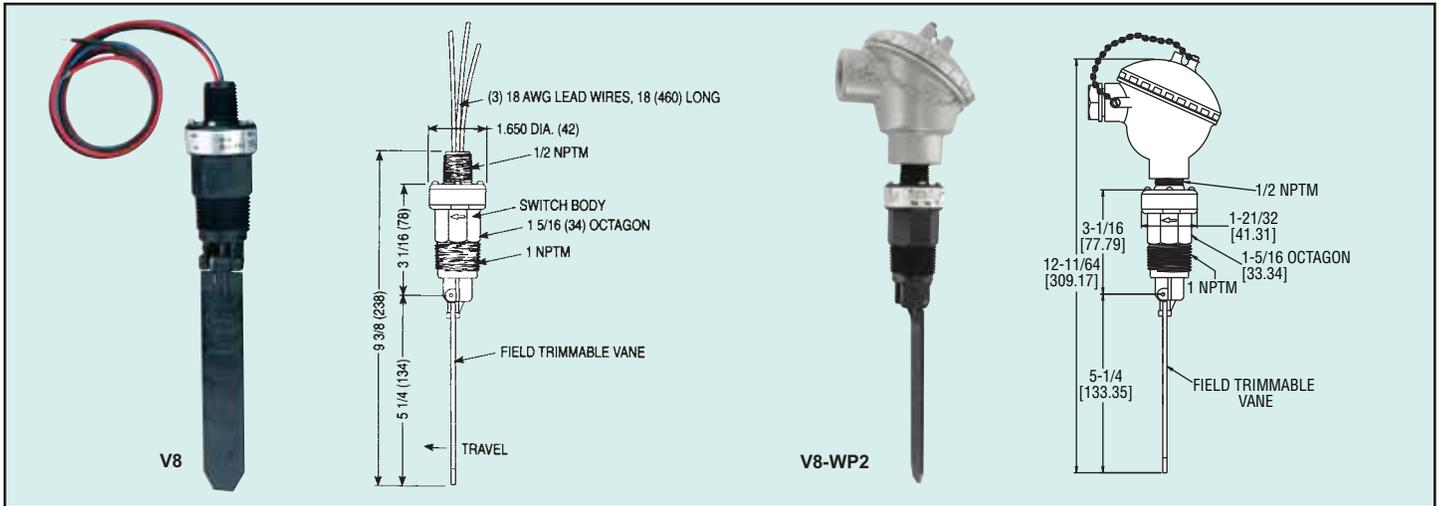
**V8 Flotect® Flow Switch Protects Equipment:** Operation is simple and dependable. In most applications, the switch is normally off while there is sufficient flow of liquid or air. When flow stops, the vane spring moves the vane, actuating a single pole double throw switch rated 5A @ 120/250 VAC to start or stop motor, pump, engine, etc. Operate a damper or valve; shut down a burner or actuate an alarm or signal, protecting unattended equipment from damage or loss of production.
