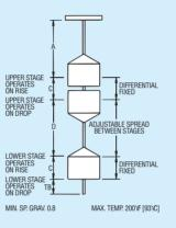
A195 - 6 Two Stage For 3" flange. Adjustable differential each stage. Lower stage operates on rise at same point upper stage operates on drop. Specific gravity 0.5 to 1.2.
