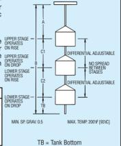
The most versatile liquid level controls in our line, displacer controls can be used to trigger alarms, provide shutdown or operate pumps.
