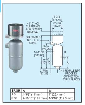
Heavy duty and low cost is the perfect description for the 391 Series level control. Stainless steel switching mechanism uses gravity return action instead of springs for long life. Weatherproof enclosure is standard. Welded steel chamber is good for 650 psig (45 bar) at 600°F (315°C).
