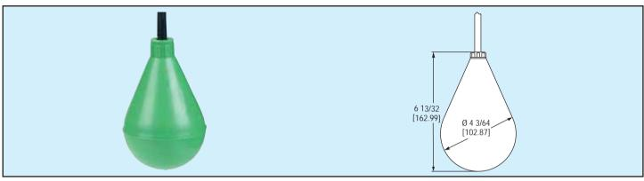
Series FSW Free-Floating Level Switch is a dual level switch designed for filling and draining of tanks, wells, and reservoirs. The shape and interior balance weight ensure impurities and dirt will not adhere to the surface, making it ideal for sewage and waste water applications. The mercury-free switch is designed with an inverter microswitch housed in a polypropylene cover.
