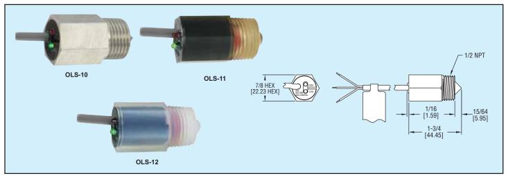
Low cost, rugged optical level switch provides rapid response while employing no moving parts for stable process control. The bright red and green LED's indicate the presence or absence of liquid for true, local indication. Three optional materials, 316 SS, polysulfone and PFA provide application flexibility. Compact switch can be quickly mounted horizontally or vertically for each installation.
