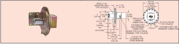
The unique electric switch design in the 1640 is another Dwyer Instruments, Inc. innovation. The Dwyer® Model 1640 Differential Pressure Switch resembles the Series 1630 switches described on the previous page. The Model 1640, however, is equipped with a single pole, double throw floating contact switch (not snap acting) so it functions as a null switch.
