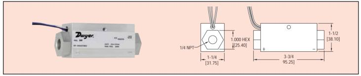
Rugged Series A4 Differential Pressure Switch offers field adjustments and can handle system pressures up to 6000 psig. Piston design allows mounting in any orientation. The switch is capable of carrying moderate shock and vibratory loads.
