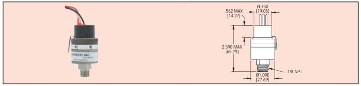
Miniature Series APS/AVS Adjustable Switches offer reliable switching for pressure/vacuum alarm, shutdown or control. The units are readily adjustable throughout their range using the locking adjusting ring and indicating pointer. The body is constructed of stainless steel for durability in harsh environments, Switches include 12" (30 cm) wire leads sealed with epoxy for additional protection.
