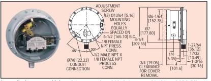
Large diaphragm sensitivity and time proven dependable design are combined in model PG differential pressure switches. Visible dial reduces "start up" time and helps prevent calibration errors. External adjustment allows set point change without removal of cover. Unit is listed by UL, FM and CSA.
