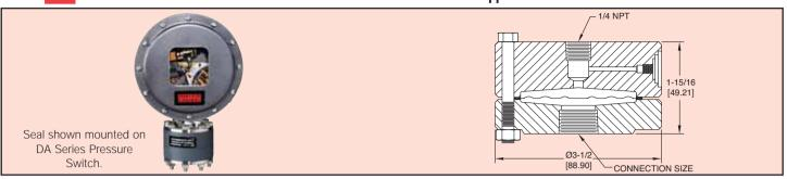
The Series XTBX is a diaphragm seal constructed of PVC and FEP making it perfect for corrosive applications that would damage metal wetted material pressure switches. The seal is available direct mounted on all model DA pressure switches with ranges under 100 psi (6.9 bar). Ideal for commercial pool/spa applications for pump shut down due to excessive vacuum.
