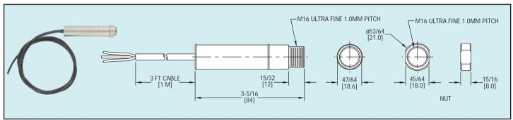
**The Series ILA Non-Contact Sensors**, measure temperatures from 32 to 932°F (0 to 500°C) and provide a linear 4 to 20 mA, 0 to 50 mV VDC or thermocouple output. The 2-wire signal is compatible with almost any indicator, controller, recorder, data logger, etc., without the need for special interfacing or signal conditioning. They are suitable for most materials such as food, paper, textiles, plastics, leather, tobacco, pharmaceuticals, chemicals, rubber, coal, and asphalt.
