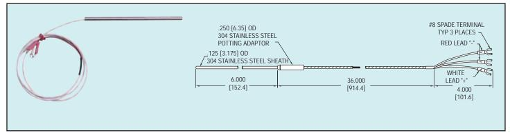
**Precision RTD** (Resistance Temperature Detector) offers excellent accuracy and stability over a wide temperature range. Industry standard 3-wire 100 ohm (DIN) probes are available in 6<sup>"</sup> (15 cm), 12<sup>"</sup> (30.5 cm), or 18<sup>"</sup> (46 cm) sheath lengths with 30<sup>"</sup> (76 cm) extension cable and spade lug terminals.
